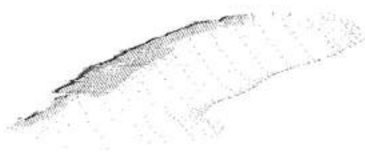
Pointset of the top of Elphinstone seam, generated from the seam pick database (8008 drillholes)
